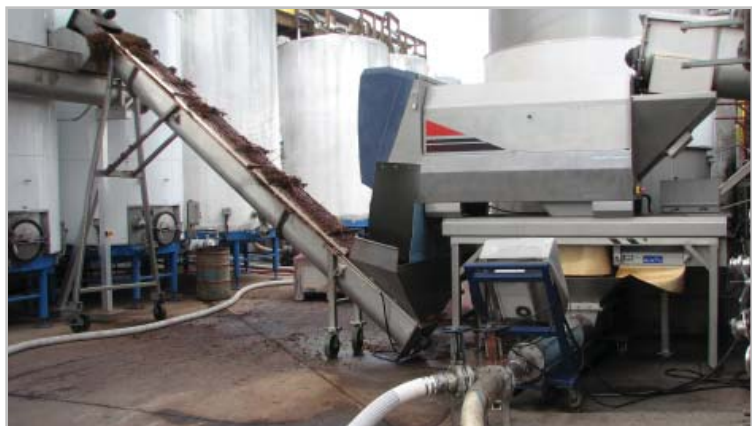
Seepex Pump below the Delta8 Crusher transferring grape MUST to fermentation tanks
