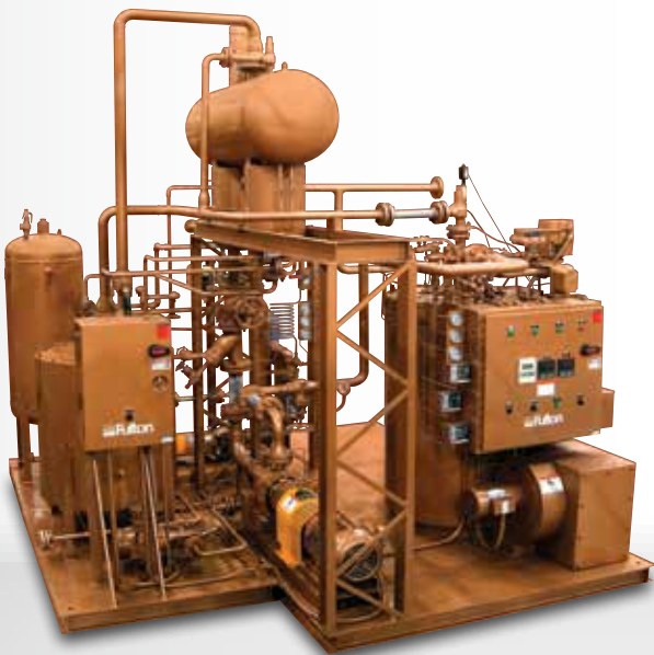
The skid system shown here included one FT-0240-C heater, a circulating pump, expansion tank and a temperature control unit (TCU). This system was designed to provide thermal fluid and hot water to several dryers for a wastewater application.
