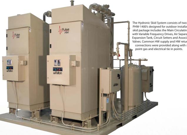
PHW-1400's designed for outdoor installation. The skid package includes the Main Circulating Pumps with Variable Frequency Drives, Air Separator, Expansion Tank, Circuit Setters and Associated Valves. Common HW supply and HW return connections were provided along with single point gas and electrical tie in points.
