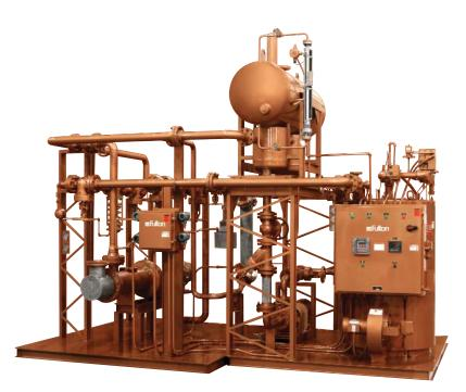
This Engineered System includes one FT-0240-C thermal fluid heater with a skid mounted circulation pump and FT-0500-L expansion tank. The system also includes two specialty heat exchangers. One exchanger uses thermal fluid to heat water, while the other heat exchanger is used to heat ethylene glycol.
