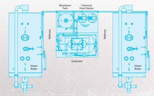
Overhead view of a pair of 250 HP Horizontal Firetube Steam Boilers skid mounted with Deaerator, Blowdown Tank and Water Treatment. Notice the custom piping to allow walkways between the boilers and accessory skid.
