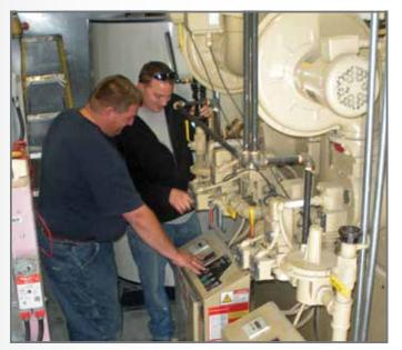
Once fabrication is complete, all units are test fired inhouse to make sure everything is operating correctly. The units are then disassembled, finished with a high quality industrial paint, and crated for shipment. Once the equipment arrives at your door, Fulton's crew of highly-trained service technicians are available to assist you with any aspect of the installation, either onsite or though our 24-hour phone line.
