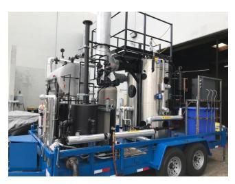
Rental and Mobile Boiler equipment is an excellent and cost effective use of temporary steam or hot water requirements.
