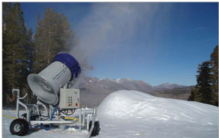
The entire underground and portable snowmaking system is fed by a single pump
