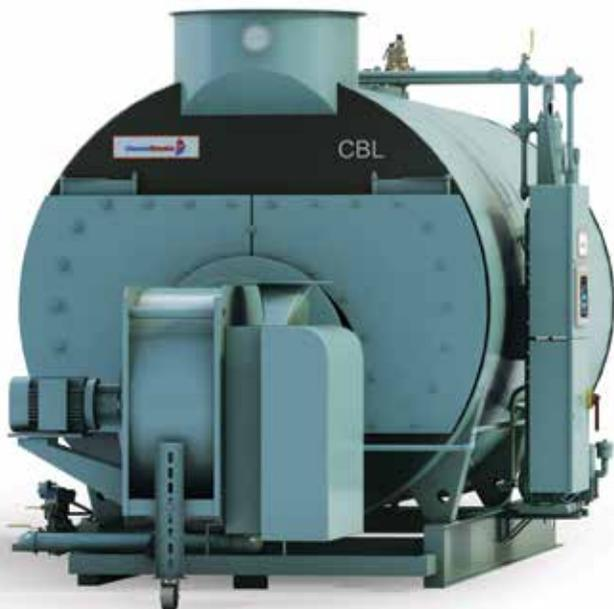
This 3- or 4- pass wetback firetube boiler is ruggedly constructed for hot water or low and high pressure steam applications. Ranging in size from 900–1,600 horsepower, this gas, #2 oil, #6 or combination fired product is a highly engineered and fully compatible boiler/burner package featuring excellent fuel to steam/water efficiency, space savings, low emissions and optional upgrades.
