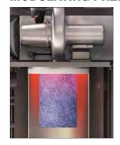
The modulating venturi premix burner and linkageless control automatically adjust the air/gas mixture for maximum efficiency and optimum turndown. A symmetrical, 360° even-temperature heat output is achieved from the burner, providing clean combustion with ultra-low NOx emissions of less than 20 ppm as standard and less than 9 ppm as optional.
